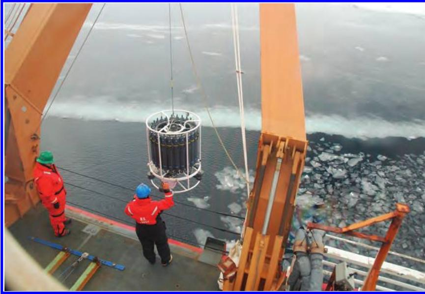
*A contraption called a Niskin bottle rosette is pulled onto the deck of the USCGC Healy, with samples from varying depths in the water column. Photograph: Lisa Robbins, US Geological Survey.*
